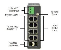
**DIN Rail Mount**: **1.** Attach the DIN Rail mounting kit to rear panel of the chassis. Insert screws and tighten then with a screwdriver to secure the kit. **2.** Insert the upper lip of the DIN rail into the DIN-rail mounting kit and press the switch towards the DIN rail until it snaps into place. **3.** Make sure that the switch is attached securely to DIN Rail.
