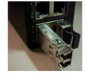
aligning it with the internal installation guides. Ensure that the SFP device is firmly seated against the internal mating connector. **4.** See the SFP manual for operating information specific to your SFP model. **5.** Connect the other end of the cable to the appropriate far end Ethernet port. After the cable is properly connected at both ends, the **SYS** LED should work.
