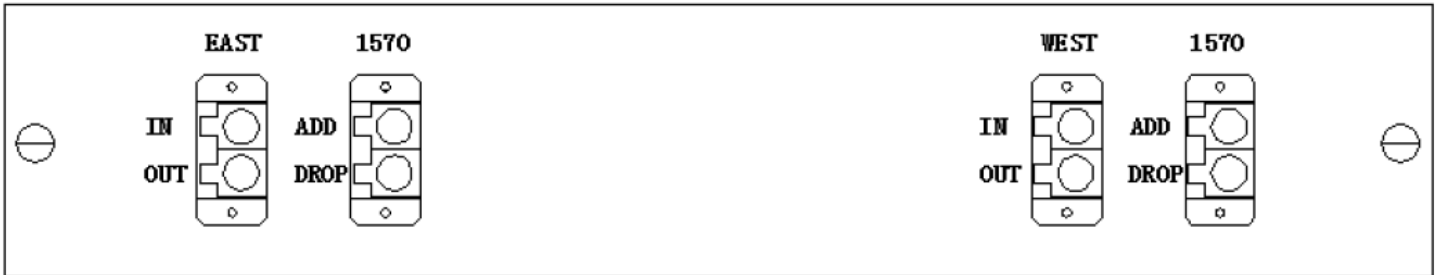
Figure 7: Add/Drop Mux Front Panel
