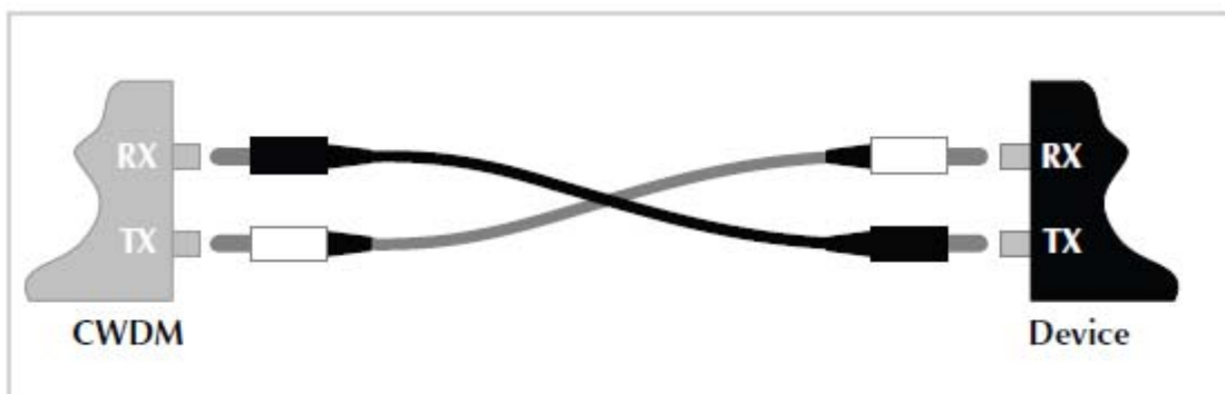
Figure 10: Fiber Cable Connections
