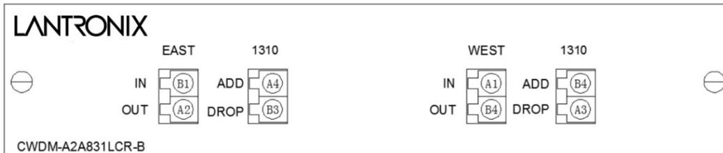
**CWDM Front Panels:** The CWDM modules have no LEDs as shown below.
