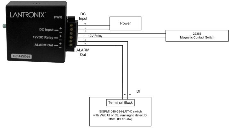
**Note**: If installing external audio or visual alarm equipment, place that equipment in series with the 22365 or with the switch that came with the cabinet.
