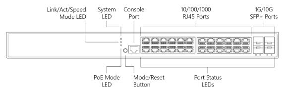
**Console Port:** The front panel Console port provides an RJ-45 Console port to connect to a PC or terminal for Command Line Interface (CLI) command entry (e.g., a PC running Hyper Terminal, Tera Term, etc.).
