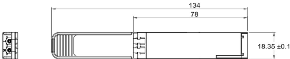
Modified TN-QSFP-100G-LR4 and TN-QSFP-100G-SR4 pull latch and unlocking structure (April 2020):
