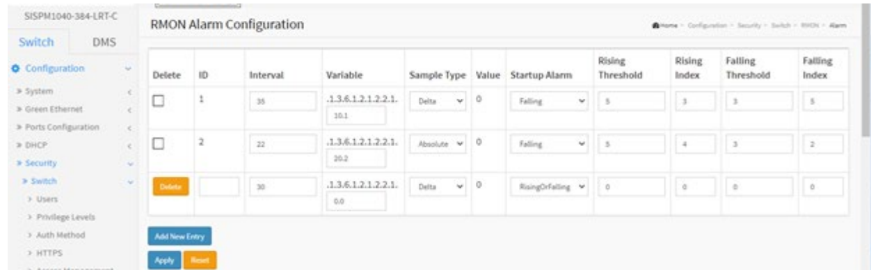
Figure 2-5.1.8.3: RMON Alarm Configuration
