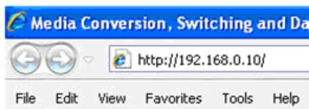
2. In the address (URL) block, type the IP address of the IONMM-232 (the default is 192.168.0.10).
