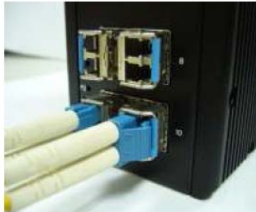
Connect the optical fiber to the SFP socket
