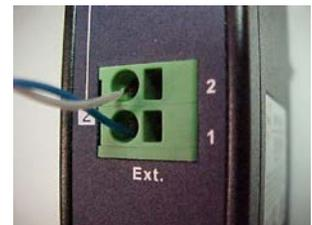
**Step 1:** Insert a small flat-blade screwdriver into the rectangular opening and insert one wire, then remove the screwdriver from the opening to secure the wire.
