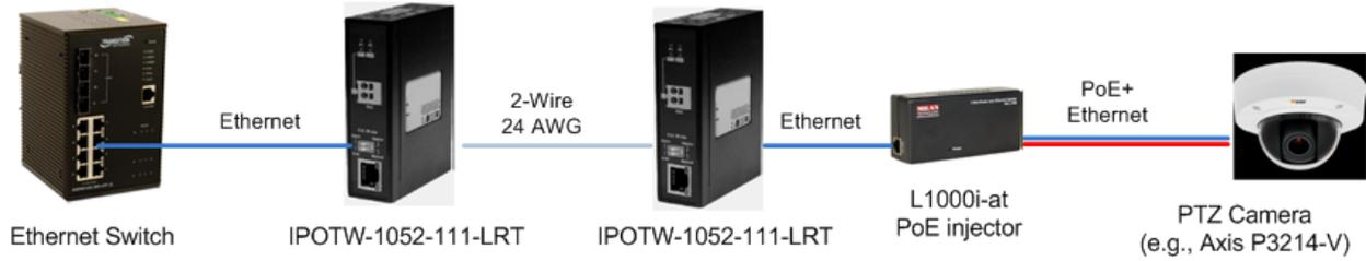
Below, two IPOTW1052-111-LRTs are used to extend the distance up to an additional 200 meters using 24AWG cable.
