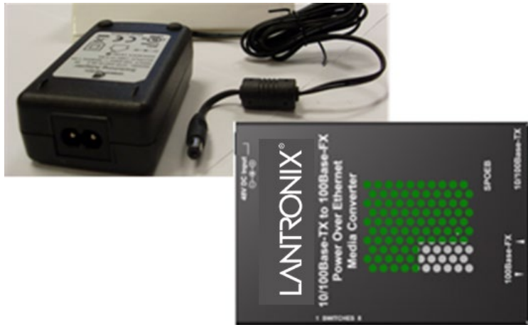
External Power Supply, Power Cord and SPOEB (included external power supply and power cord may vary by region)
