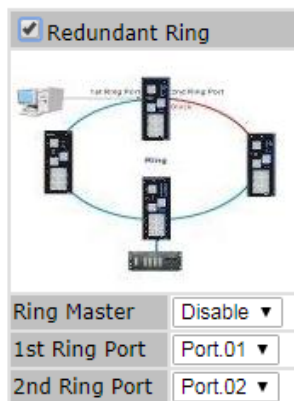
Redundant Ring interface
