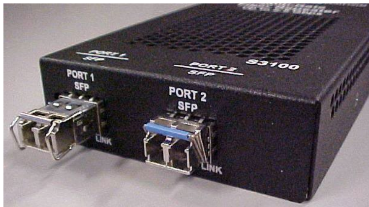
Figure 3: Port Locations and SFP Installation
