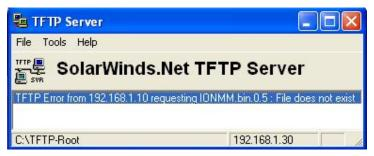
**Meaning**: A TFTP Server error - the TFTP Server Address that you specified does not contain the Firmware File Name specified.
