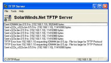
Meaning: A TFTP Server error - you tried to upload a file e.g., (IONMM.bin.0.5 – 50Mb) but the TFTP server failed. The file you tried to upload via the TFTP server exceeded the file size capability.
