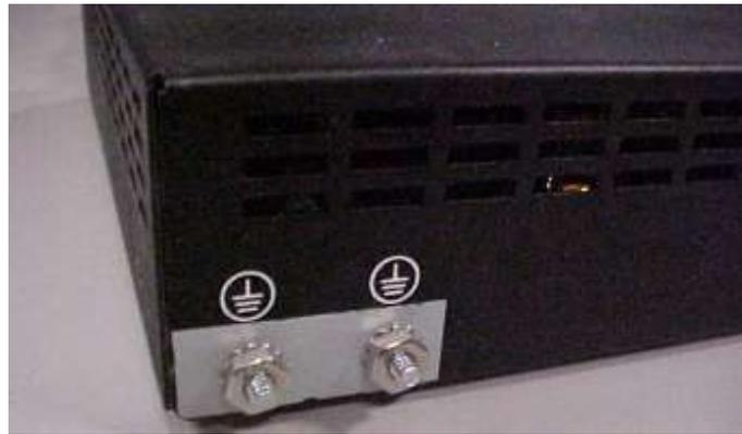
**Figure 11: C. GND (Chassis Ground)**
