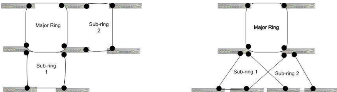
Figure 10. Multiple Sub-rings connected to a Major Ring
