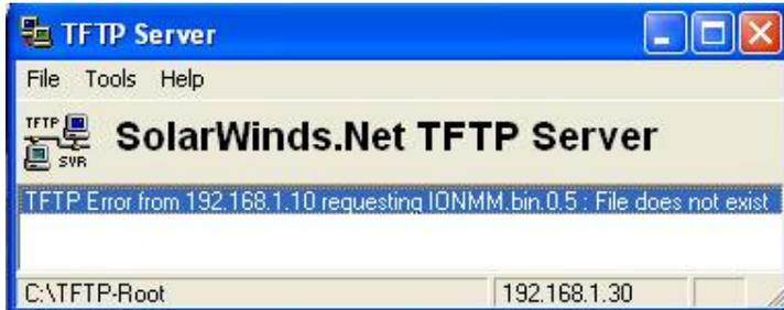
**Meaning:** A TFTP Server error - the TFTP Server Address that you specified does not contain the Firmware File Name specified.
