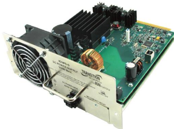
Figure D-3: IONDCR Installed in IONPS-D (DC) Power Supply
