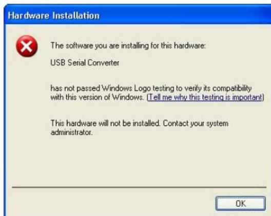
To successfully install the device, you must change the driver signing options to either warn or ignore to allow the installation to complete.
