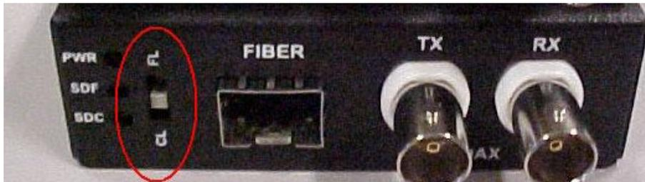
**CL / FL Switch SW1** - Loopback test mode:
