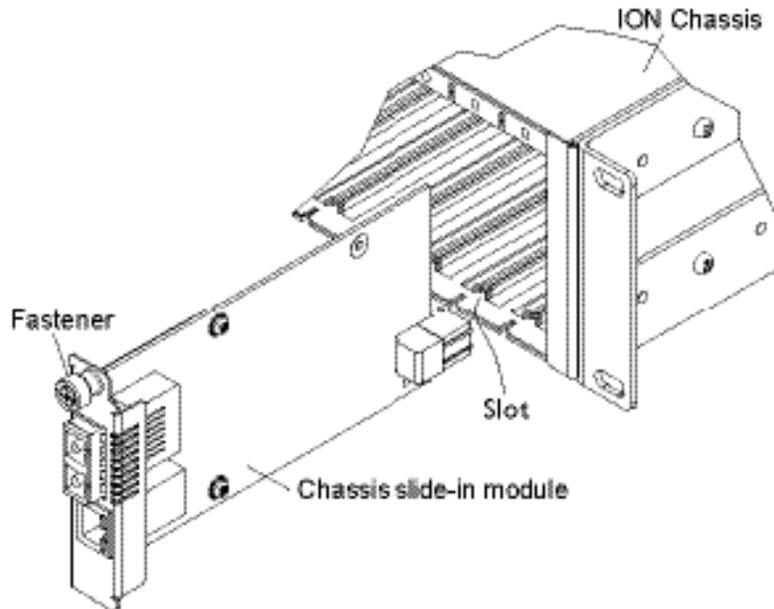
3. Loosen the panel fastener by turning it counterclockwise.
