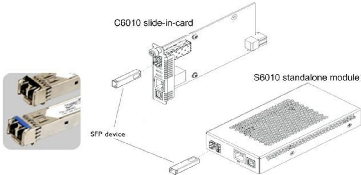
**Figure 17: SFP Installation**
