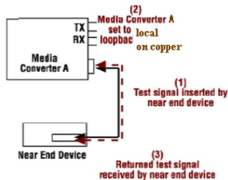
Figure 5: Typical Loopback function on a Copper port
