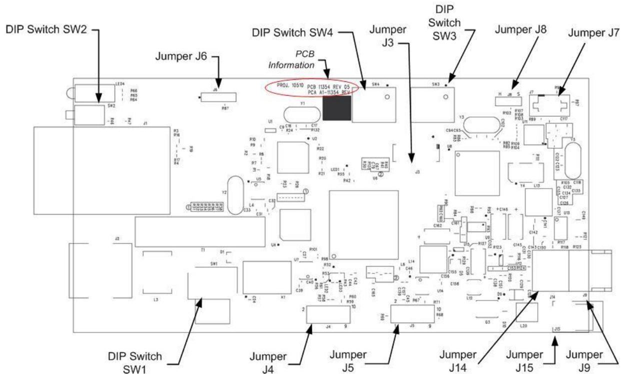
**Figure 19: x6010 PCB Layout**
