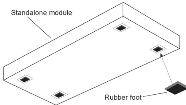
**Figure 14: Tabletop Installation**
