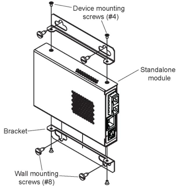
**Figure 15: Wall Mount Installation**
