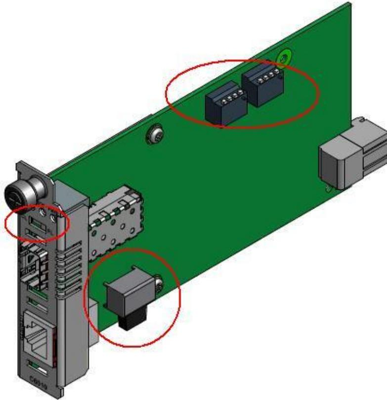
Figure 12: C6010 DIP Switches
