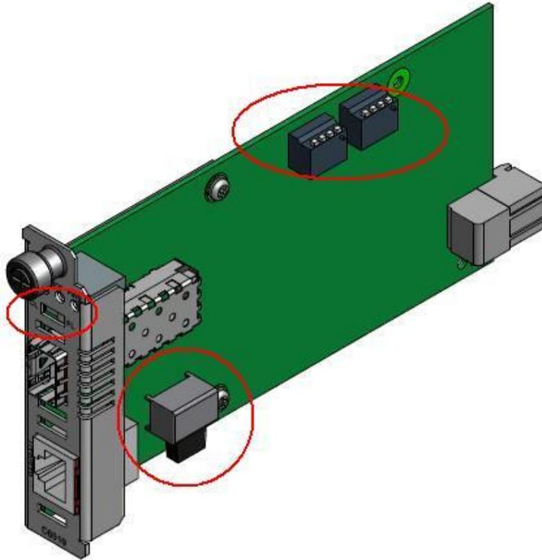
Figure 12: C6010 DIP Switches
