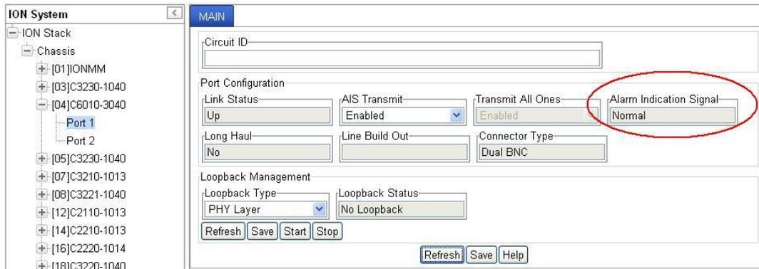
5. Verify that the **Alarm Indication Signal** field has changed from **Alarm** to **Normal**.
