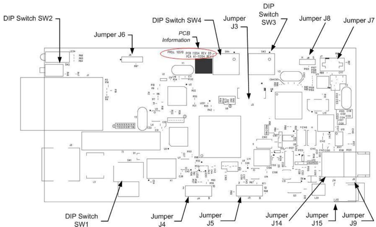
**Figure 19: x6010 PCB Layout**
