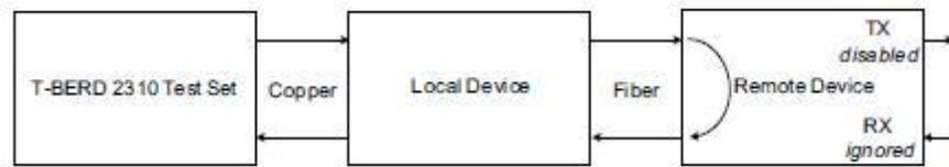
**Figure 22: Initiate a Loopback from a Test Set**
