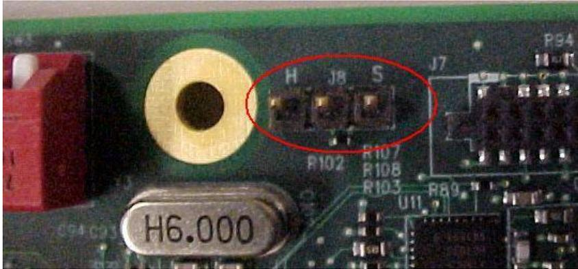
The J8 factory default setting is Software mode (pins 2 and 3 jumpered) as shown above.
