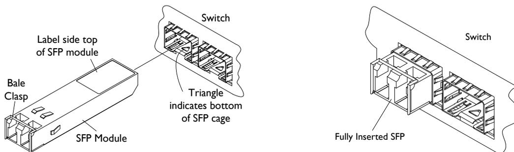
6. Ensure that the SFP device is firmly seated against the internal mating connector. To verify that the SFP is seated and latched properly:
