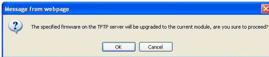
8. Click **OK**. The upgrade begins and the message *"the firmware is being upgraded"* displays. The Status field displays *"Success"* when the firmware upgrade successfully completes.
