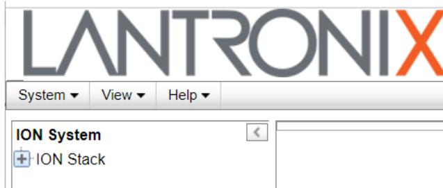
7. Click the plus sign **[+]** next to **ION Stack**. This unfolds "ION Stack" node in the left tree view and will refresh device status.
