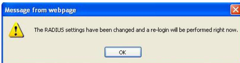
**Meaning:** You performed a Copy Certificate function for the IONMM in the RADIUS tab.
