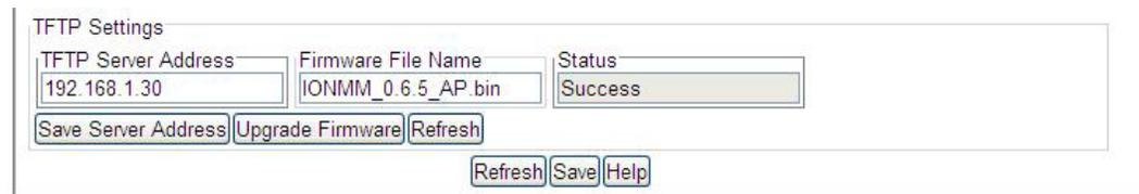
If the upgrade fails, the message *"The firmware upgrade failed!"* displays. Click the web page **OK** button to clear the message. (If the **Status** field displays the reason *"TFTP Failure"*, make sure the TFTP server is running and properly configured.)
