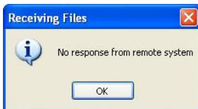
You entered a Serial File Transfer command, but the ZModem file transfer failed.
