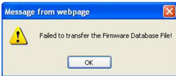
**Meaning:** While performing a Firmware Upgrade from the **MAIN** tab > **TFTP Settings** section, a problem was detected. See the [Upgrade the IONMM Firmware](#) section.
