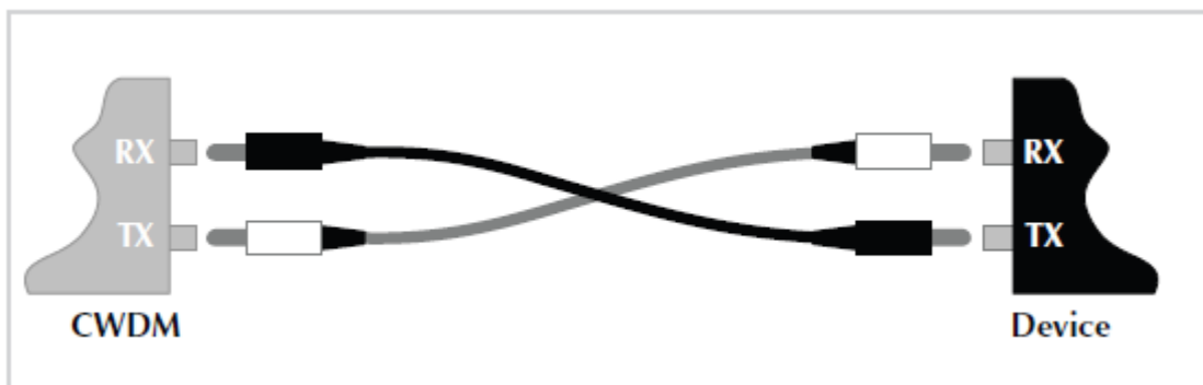
Figure 7: Fiber Cable Connections
