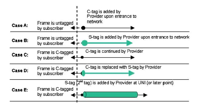
Note: Using Case A above, Port-1 is facing the untagged customer traffic and Port-2 is facing the service provider. The traffic from the customer (copper port) will egress out tagged in the provider (fiber port) and vice-versa in the opposite direction.
