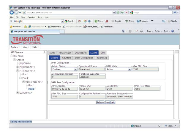
If provisioning the standalone S323x NID for remote operation without ION management, by default, the S323X is managed by the ION Management Module. Setting the mode to **local** indicates that the device is not managed by the ION Management Module but either a direct USB connection or a direct network connection via Telnet or the Web interface. Setting the mode to remote indicates that the device is managed through the ION Management Module.
