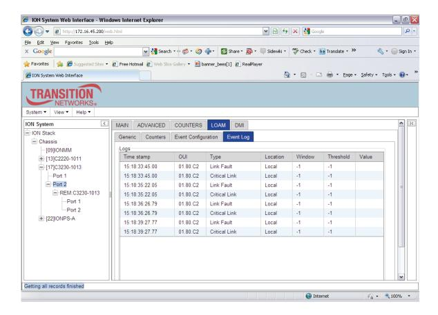
To remotely managed specific OAM critical events, set up SNMP trap host managers in the ION management module (see App. Note ###) for set-up instructions.
